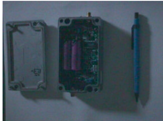
Figure 2: Logic control and data storage unit.
