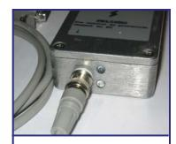
A BNC coax connection allows downloading the acquired information. An Interphase cable supplied with the kit is including a BNC terminal for the ILMOS acquisition box in one end, and a DB9 terminal to be plugged into the computer in the other.
